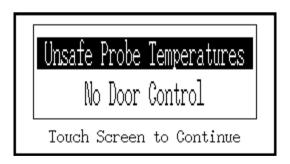
If the chamber temperature is above the pre-set maximum for a cycle, then the door will be prevented from opening, even if the cycle has successfully completed sterilization.
