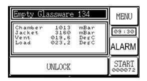
The '**Unlock'** button starts the unlocking sequence and one of the following screens will appear whilst door unlocking is in progress:
