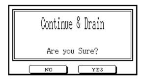
Saying Yes to this confirmation will require a Supervisor or above level password. If a valid password is entered, the cycle will go through the pre-determined fault stages of the cycle as if it was not a discard cycle, dumping the effluent down the drain and completing the cycle with door control available.
