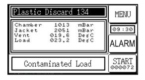
This screen will occur if the chamber is sealed because a discard cycle has failed and the chamber contains contaminated waste. The cycle must be run again and pass before door control is possible.
