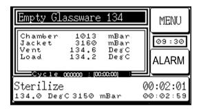
In the cycle status display, information about the current stage in progress within the cycle and the stage and cycle times is displayed.
