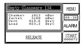
When the Autoclave is in cycle, the door control buttons and cycle control area is replaced by a cycle status display.
