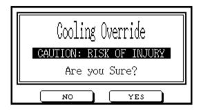
By touching the **YES** button, the autoclave will move to the next stage in the cycle. When the cycle has finished, the User will be warned that this function was used and will not be permitted to move on to door control until the User's password has been entered. Door control will continue to be restricted until the temperature is below the temperatures specified in the cycle parameters.
