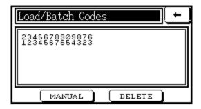
If a barcode scanner is attached, simply scan in the barcodes. Touch the '**Delete'** button to delete the last code entered.
