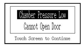
If the chamber pressure is below the pre-set minimum for a cycle, then the door will be prevented from opening, even if the cycle has successfully completed sterilization.
