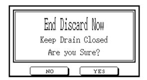
Saying **Yes** to this confirmation will end the cycle immediately and move to the 'Failed' Screen. The chamber will remain sealed. Door Control will not be available and it will be impossible to select a different cycle. To clear this problem, run the discard cycle again. Once this has completed successfully, normal control will be available.
