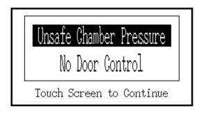
If the chamber pressure is above the pre-set maximum for a cycle, then the door will be prevented from opening, even if the cycle has successfully completed sterilization.
