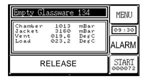
Touching the 'Release' button to allow the door to open.
